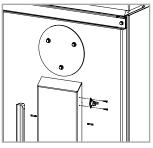
Remove the rear side with the size 8 key (M5 screws), take the contact thermostat from the kit box and connect it to the side of the air duct using a Phillips screwdriver.
