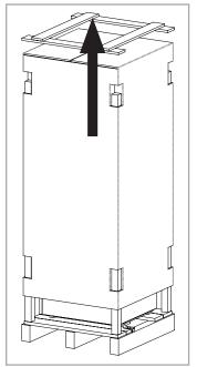
The body must always be moved in a vertical position using trolleys.
