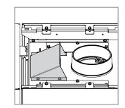
Lift the cast iron top and fix the air conveyor with the size-8 key (M5 screws).
