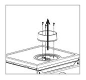
Remove the rear pre-drilled hole to gain access and remove the cap, unscrewing the 3 screws with the size 8 hex key. Repeat the operation to remove the cast-iron collar fixed to the product head.
