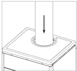
ATTENTION TO THE SECTION OF THE SMOKE DUCT WHICH MUST WIDHSTAND TEMPERATURES THAT CAN EASILY REACH 600°C. NEGATIVE PRESSURE IN THE SMOKE EXHAUST SYSTEM MUST RESPECT THE VALUE OF 11Pa.
