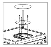
With the 3 M5 screws, fix the collar where the cap was previously removed and connect the horizontal section of the smoke duct;
