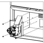
Following the holes (see arrows), fix the ventilation kit to the internal rear plate with a size 8 key (M5 screws).
