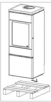
To remove the appliance from the pallet, unscrew the metal supports holding it, so as to release it from the wooden base.
