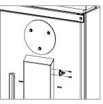
Remove the rear side with the size 8 key (M5 screws), take the contact thermostat from the kit box and connect it to the side of the air duct using a Phillips screwdriver.
