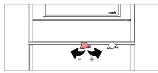
To verify proper combustion, check the colour of the flame. If the flame tends to darken, generating soot in the combustion chamber and black puffs of smoke, this is an indicator of bad combustion due to lack of air. It will therefore be necessary to add secondary air by turning the central lever to the right (+) to improve combustion.
