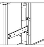
For models equipped with drawer, it is necessary to remove the drawer before installing the kit by acting on its rails with the 2.5 wrench (M4 screws).
