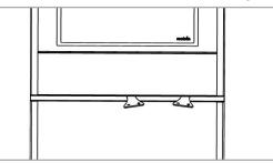
Combustion is efficient and "clean" when the flame looks pale yellow. If the flame tends towards red, or if you notice black smoke in the combustion chamber, turn the handle in the middle to slightly increase secondary air.
