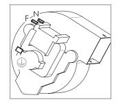
Remove the pre-drilled grid to allow the wiring to pass from the contact thermostat to the air fan (see wiring diagram at the end of the manual for further details).
