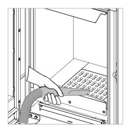
Extract the drawer under the grate of the combustion chamber and empty it, paying close attention for the ash could still be incandescent.
