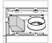
Lift the cast-iron top cover and fix the air conveyor with the size 8 key (M5 screws).
