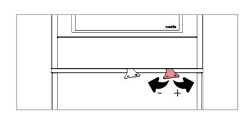
The central handle controls secondary air and is used to adjust combustion when the stove is running. Secondary air is fully open when the handle is turned to the right (+), while it decreases when the handle is moved to the left (-).
