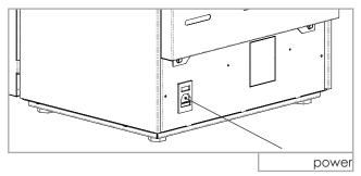
It is mandatory that the system is equipped with both earthing and differential switch, as per the laws in force. Also, make sure that the socket is compatible with the type of plug on the power cord used.
