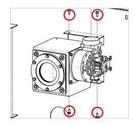
Take the ducting cover out of the packaging again and, using the 4 fastening screws (already present and screwed onto the product body), fasten it as shown in the figure.
