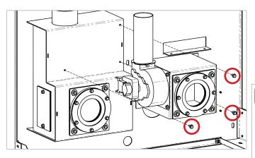
Take the ducting cover out of the packaging again and, using the 4 fastening screws (already present and screwed onto the product body), fasten it as shown in the figure.
