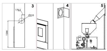
**3** Using the positioning and sizing measurements, prepare the gap in the plasterboard to secure the loading system.
