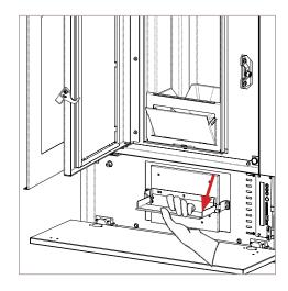
Remove the ash pan and empty it, as in the figure below:
