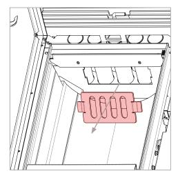
With a soft bristle brush, eliminate the combustion particulate, allowing it to fall in the slide beneath.
