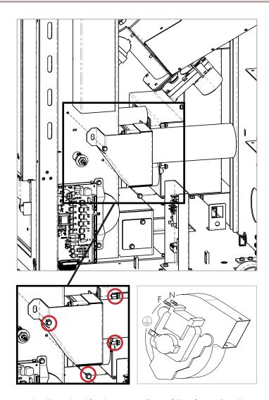
Make the electrical connection of the fan using the CANAL appendix, already present in the original wiring of the product. Live and Neutral can be inverted, unlike the earth connection (yellow / green colored cable) which must be connected to the earth of the fan.
