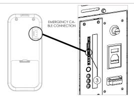
Before connection using the emergency cable, remove the batteries from the handheld device from the specific compartment. DANGER OF FIRE
