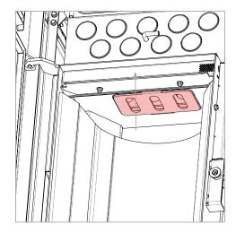
Remove it by bringing the lever towards you with slight movement downwards as in the figure below:
