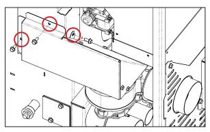
Make the electrical connection of the fan using the CANAL appendix, already present in the original wiring of the product. Live and Neutral can be inverted, unlike the earth connection (yellow / green colored cable) which must be connected to the earth of the fan.
