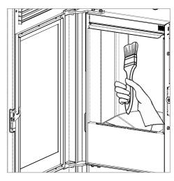
Vacuum the slide, the hatch and the surface hidden by the flame trap, paying attention not to knock the vacuum cleaner nozzle off the vermiculite.
