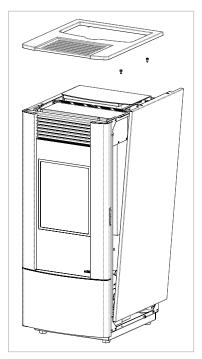
Position the stove canalization adapter by means of the 3 screws 5, present in the kit, and an 8mm hexagonal wrench.
