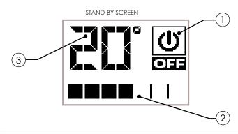
After 20 seconds of inactivity, the display on the handheld device blacks out and passes to "SLEEP" mode, maintaining the remote connection with the appliance. The display re-enables only by pressing the (1) key.
