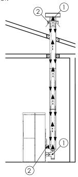
For coaxial installation or air sampling directly from the outside, it is recommended not to exceed 2.5 / 3 linear meters in order to ensure correct oxygen supply to combustion.
