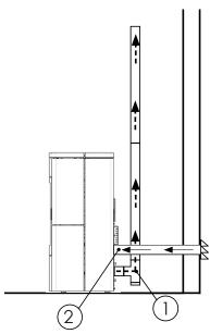
smoke discharge (1) and oxidising air channelling
