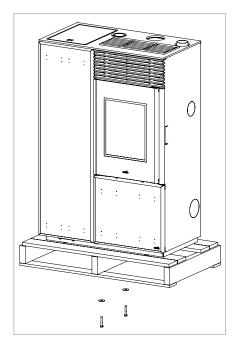
Position the equipment and proceed with its connection to the chimney flue. Find, using the 4 adjustment feet, the right level so that smoke discharge and the pipe are connected correctly.
